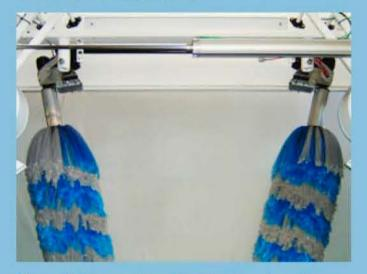
The oscillating system of vertical brushes, allows them to work in a uniform manner, over the entire lateral surface of the vehicle, since the support is guaranteed only by their weight.
