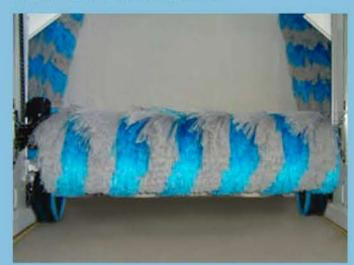
The horizontal brush is controlled by an amperometric electronic system which ensures maximum reliability.
